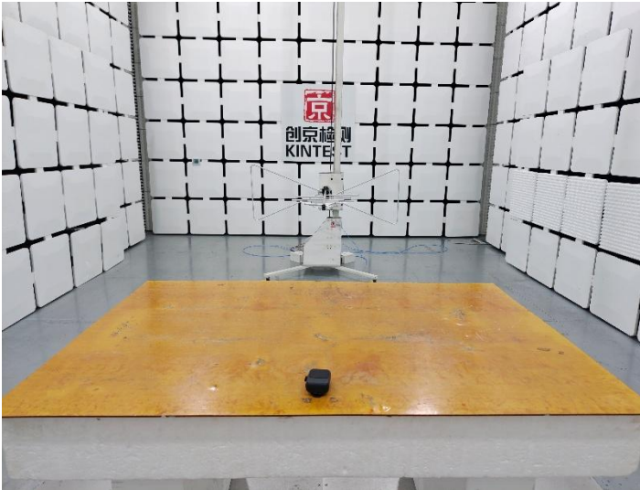
Radiated electromagnetic disturbances (30 MHz to 1000 MHz) Mode 1
